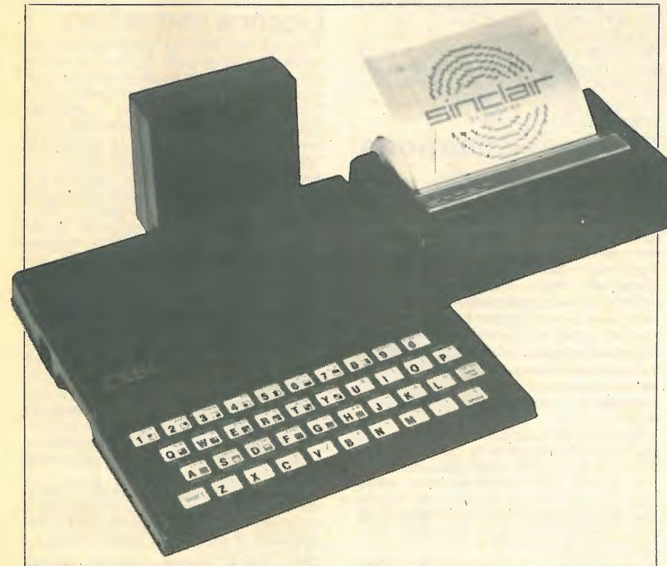
The Sinclair ZX81 which is to be manufactured, and marketed in North America, by Timex. The ZX81 is shown together with the add-on 16K RAM pack and the ZX Printer.
